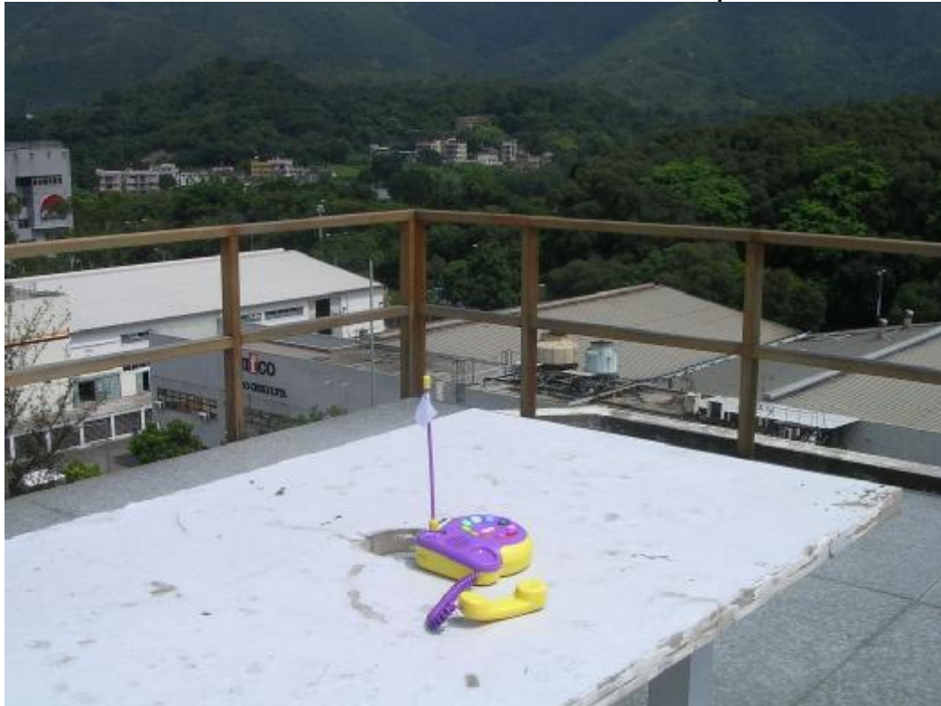
Measurement of Radiated Emission Test Set Up
