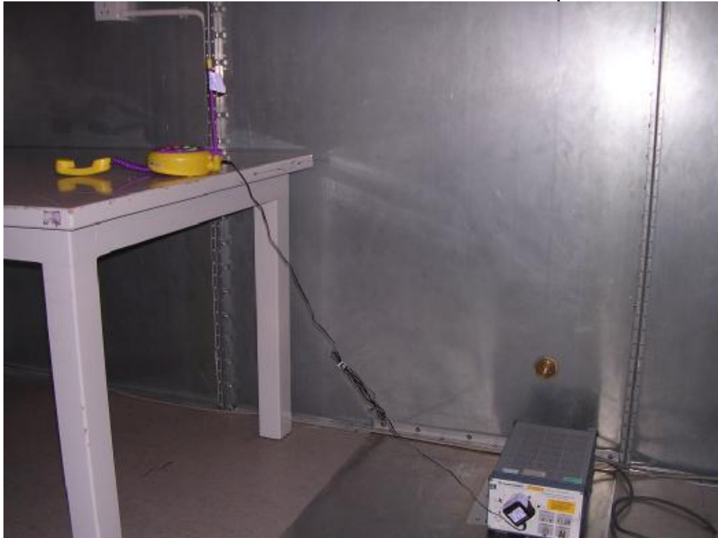
Measurement of Conducted Emission Test Set Up
