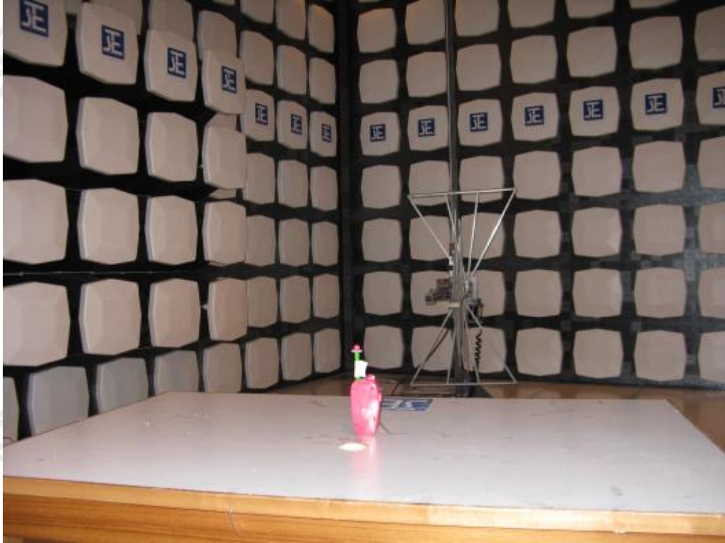
Measurement of Radiated Emission Test Set Up
