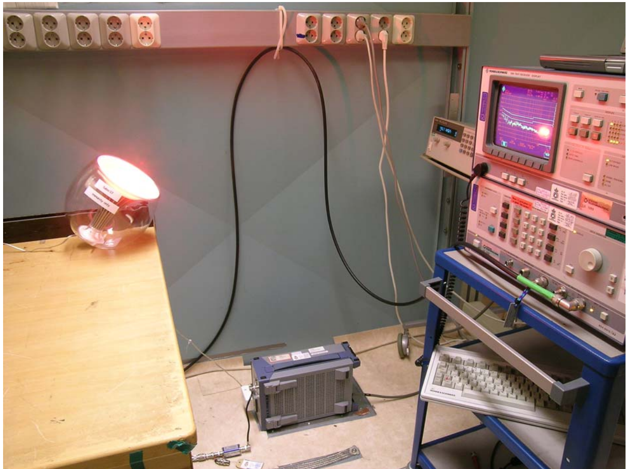
Power Line conducted emission test
