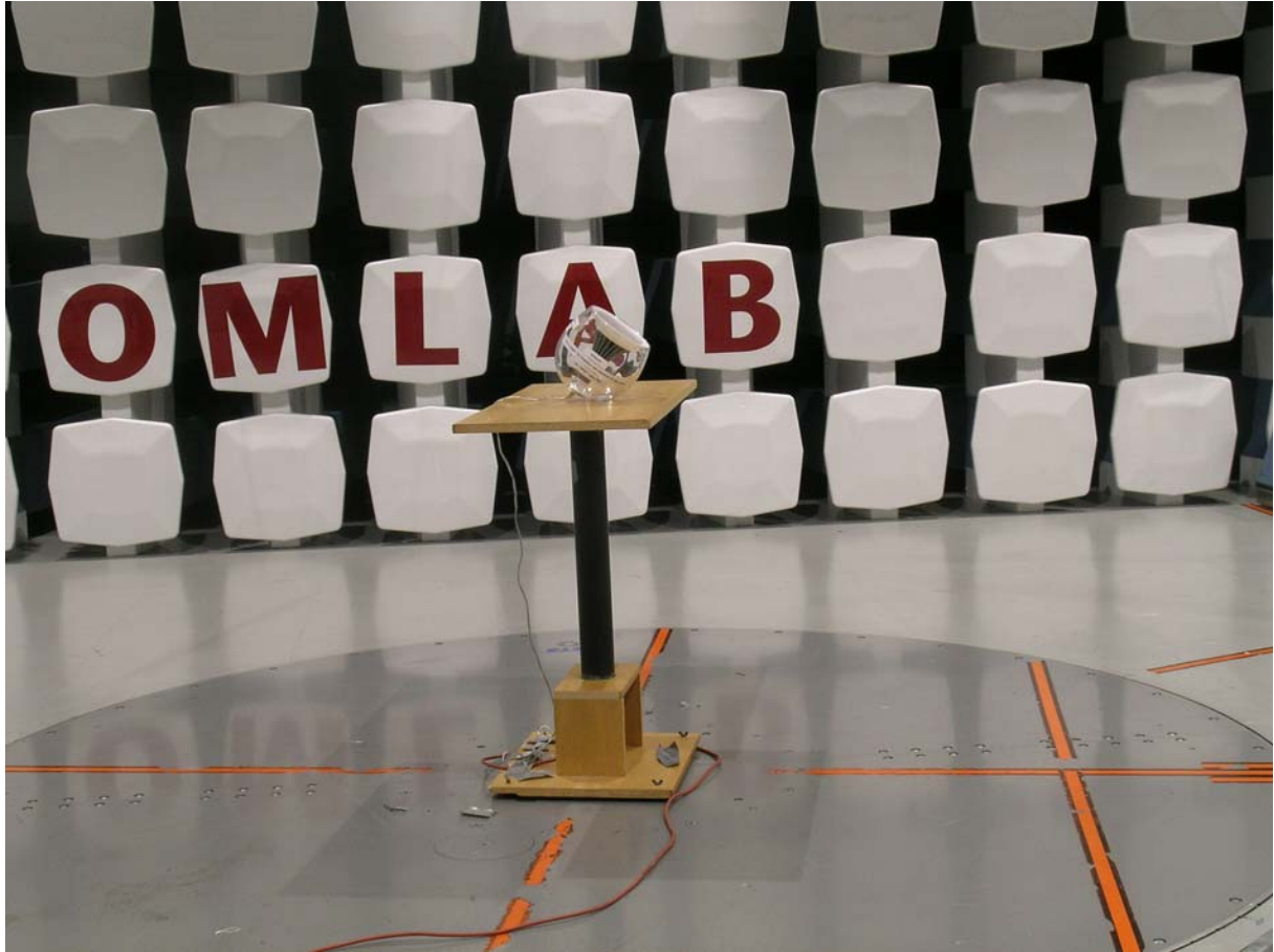
Radiated emission 9kHz – 25 GHZ
