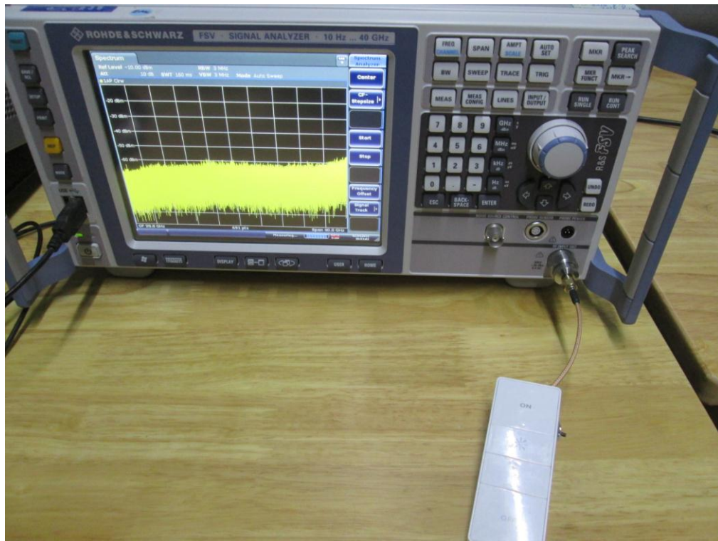
Figure 2 Conducted measurement Test setup
