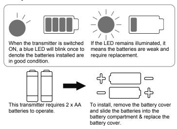
Note: Batteries contain a corrosive acid that may leak and damage the transmitter when stored for a long period. Batteries should be removed from the transmitter before storing without use for more than 4 weeks.
