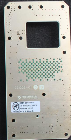
SCV-A113 Downconverter PCB 001335-3 (underside)
