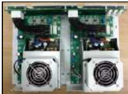
Radar Distribution Unit Power Supply
