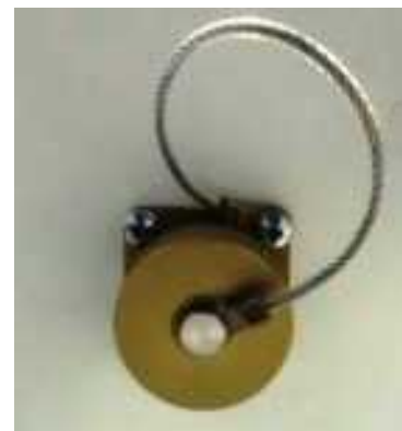
Detail of fibre connector on base of enclosure
