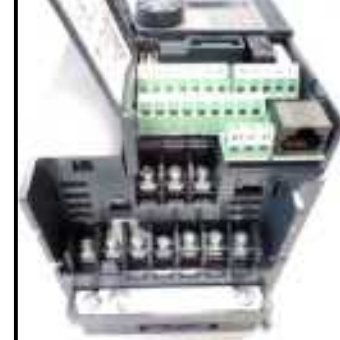
Lower terminal protection cover fitted (left) and removed (right).
