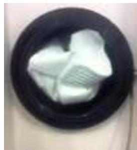
Example of desiccator with cover removed
