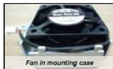
Fan showing retaining screw and power connection
