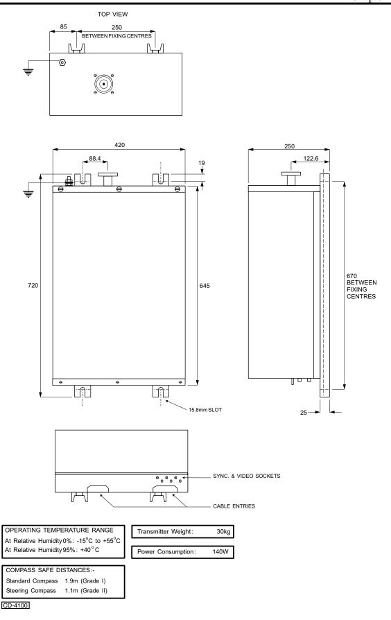
Figure 1 - Downmast Transceiver (CTX-A9): Installation Dimensions
