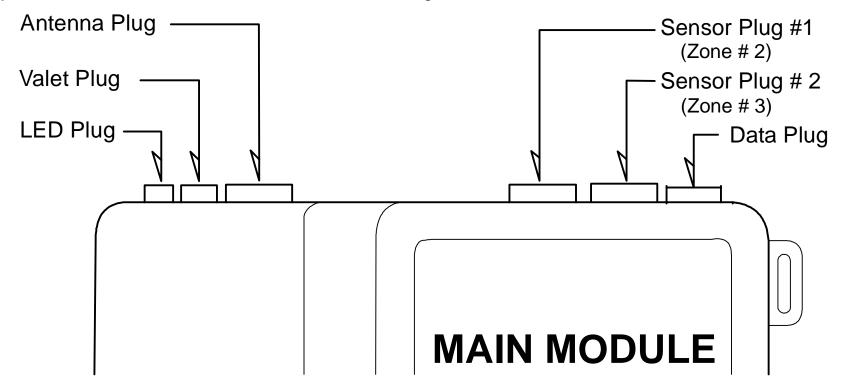
The Sensor Plug #2 is zone 3 for an optional sensor.
