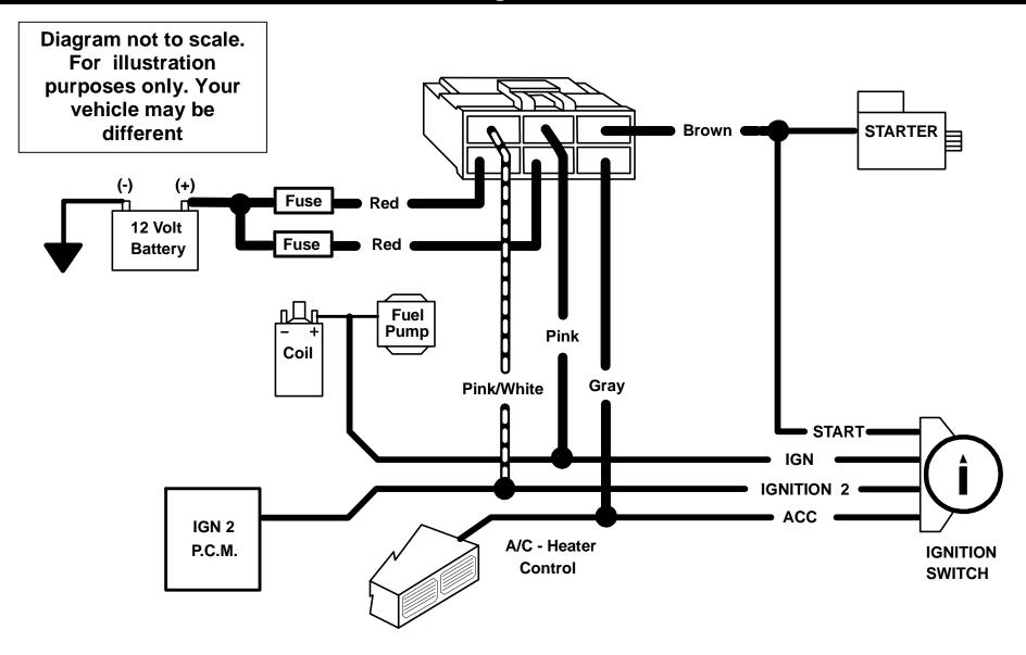
NOTE! Use External Relays for High Current Ignition and/or Accessory circuits greater than 30A. Failure to do so could result in damage to the unit that is not covered under warranty. \*\*\*\* Fuse Holders Wire Connections should NOT GET HOT \*\*\*\*
