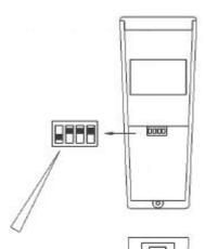
Press firmly below arrow and slide battery cover off.
