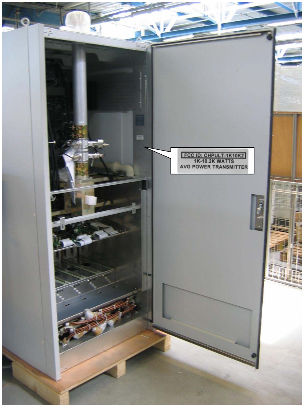
Figure 2 Label placement on transmitter cabinet
