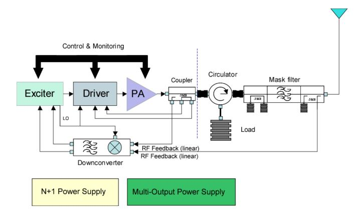
Simplified Transmitter Block Diagram
