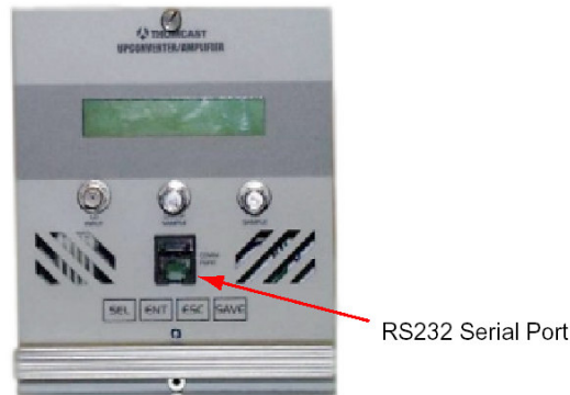
Figure 1 Upconverter RJ11 Serial Port Connector
