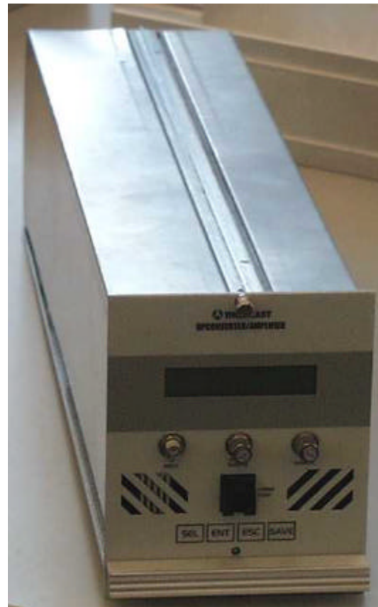
Figure 1: Upconverter plug-in module.
