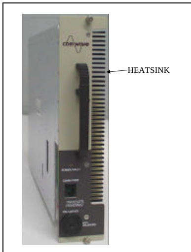
Figure 2: Power amplifier segment heatsink.
