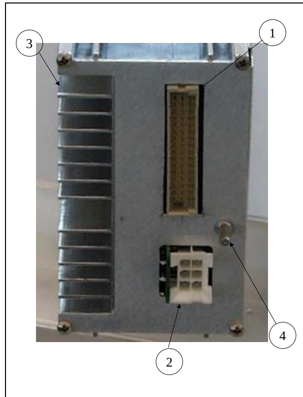
Figure 3: Power supply module rear panel.
