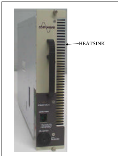
Figure 2: Power amplifier segment heatsink.
