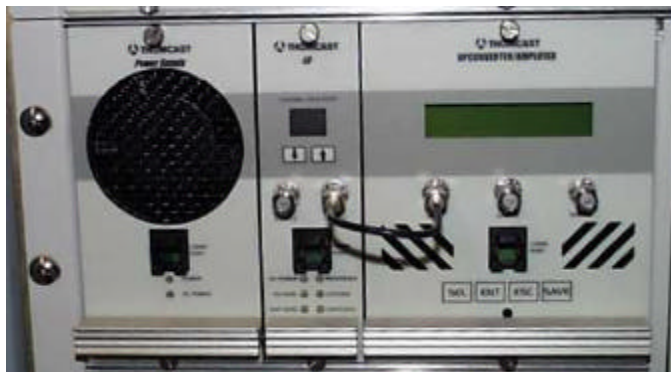
Figure 1: Cabling the LO signal.
