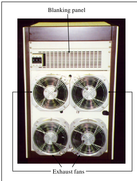
Figure 13: Blanking panel & exhaust fans.
