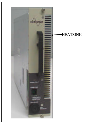
Figure 12: Power amplifier segment heatsink.
