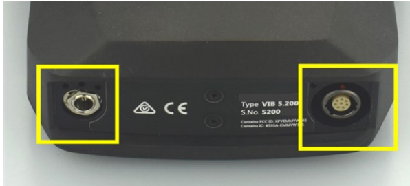
Charge socket (left) and multipole analog measuring channel (analog IN, right) at the bottom of the device.
