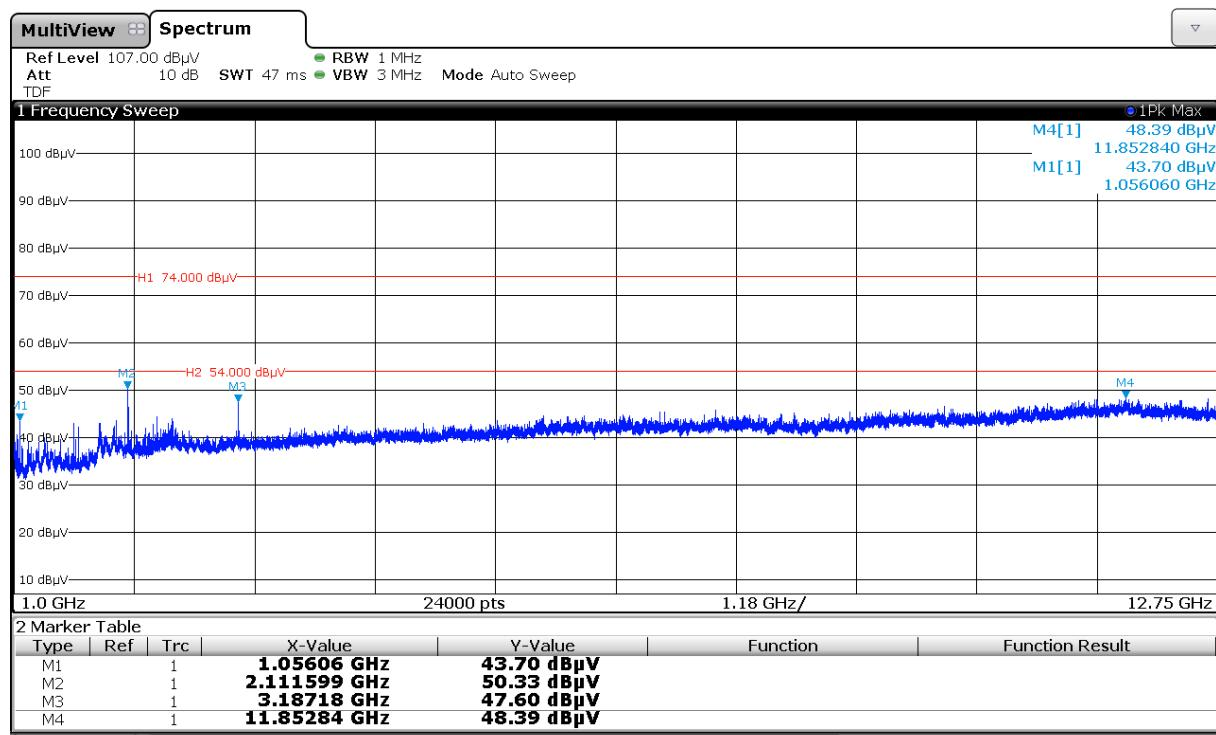
Note: The peak values fulfil the average limit, therefore an average measurement is not necessary.
