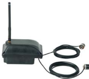
Sensor unit with two sensors, for vibration and temperature measurement respectively.
