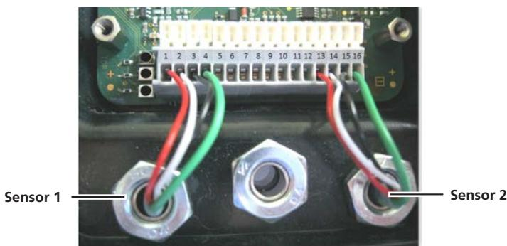
Sensor 1 (left) is assigned to channels 1 and 3.
