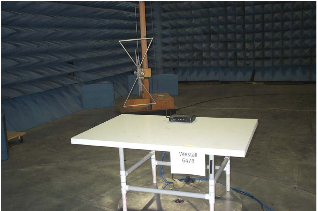
Photograph of Conducted Emissions Test Setup
