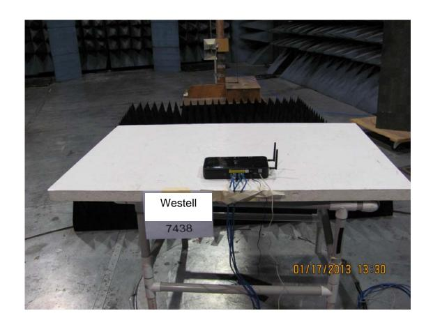
Photograph of Conducted Emissions Test Setup
