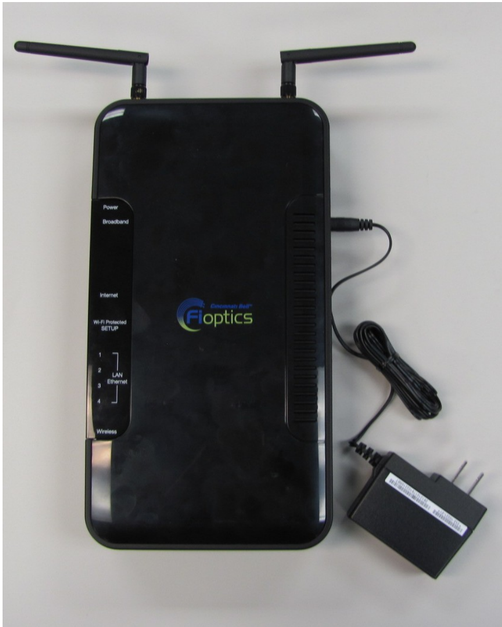
Top of Gateway Modem Case with power supply connected
