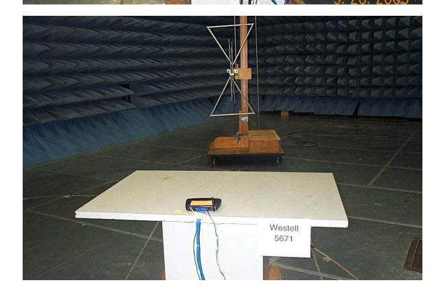
Photograph of Conducted Emissions Test Setup
