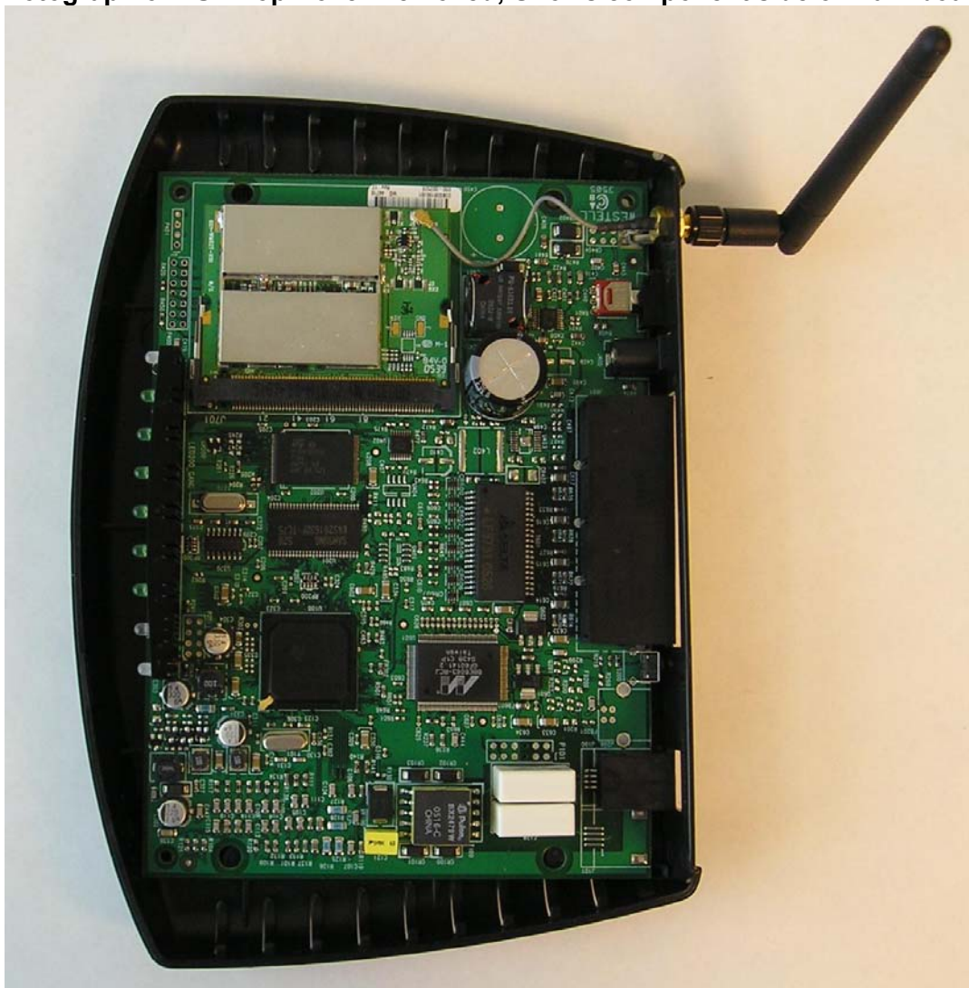
Photograph of EUT-Top Cover Removed; Shows component side of Main board
