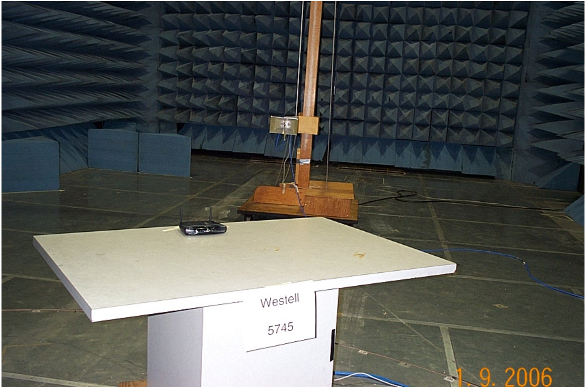
Figure 3. Photographs of Radiated Emissions Test Setup
