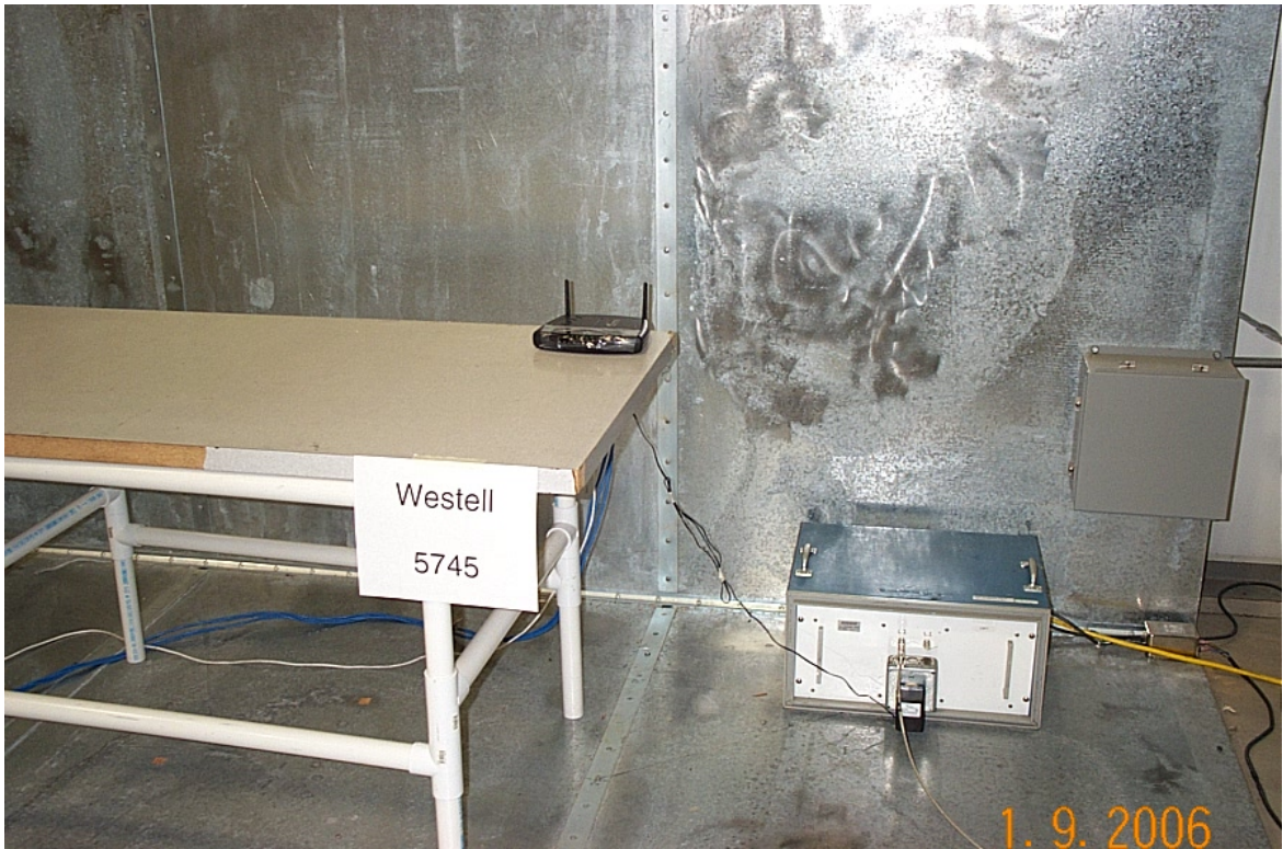
Figure 4. Photographs of Conducted Emissions Test Setup
