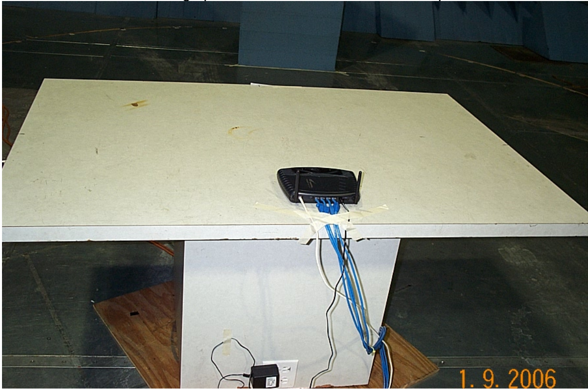
Photograph of Radiated Emissions Test Setup
