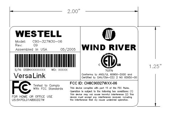
The label will be on the bottom center of the unit. The label is compliant to UL 60950 Section 1.7.13 Durability of Markings.
