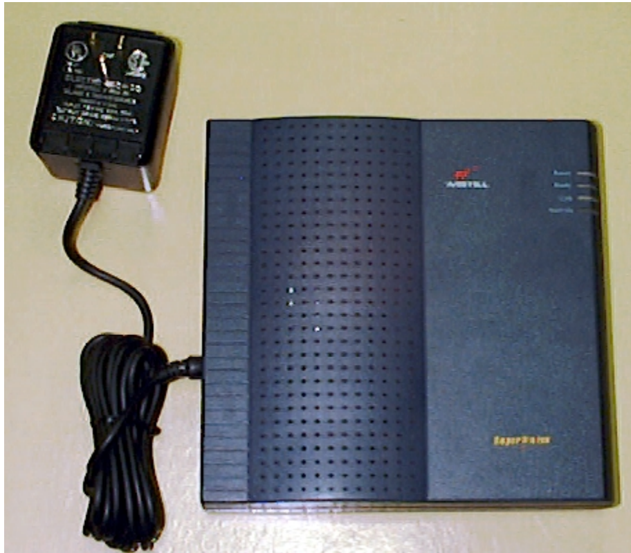
Top of EUT showing AC-AC power supply
