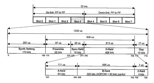
The basic, repeating, frame structure is 10 ms long. It is sub-divided into 8 slots, each 1250 µs long. The active transmission time is 937.5 µs. The first 4 slots form the 'up-link', when the PPs transmit to the FP. The last 4 slots form the 'down-link', when the FP transmits to the PPs.
