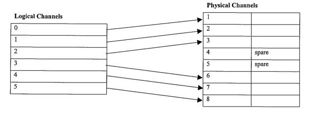
Noisy channels can be adapted out of the sequence by 'channel swapping', i.e. swapping a good spare channel for a noisy channel. For example, swapping physical channels 1 and 3 gives:
