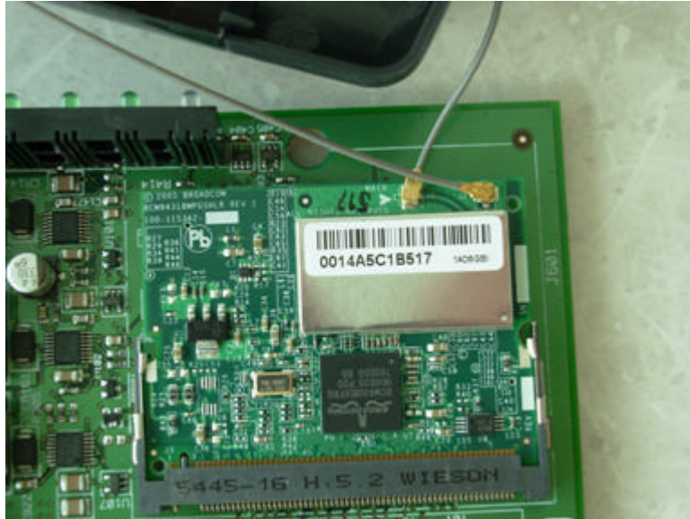
Photograph showing connection from WiFi board to antennas
