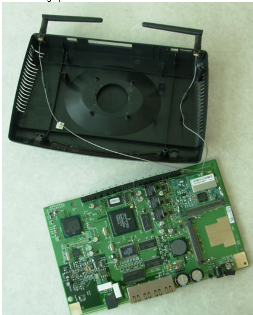
Photographs of connections from the board to antennas
