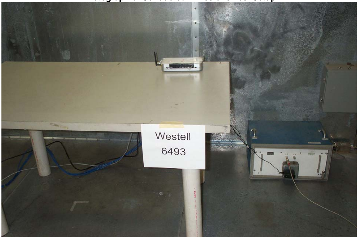
Photograph of Conducted Emissions Test Setup
