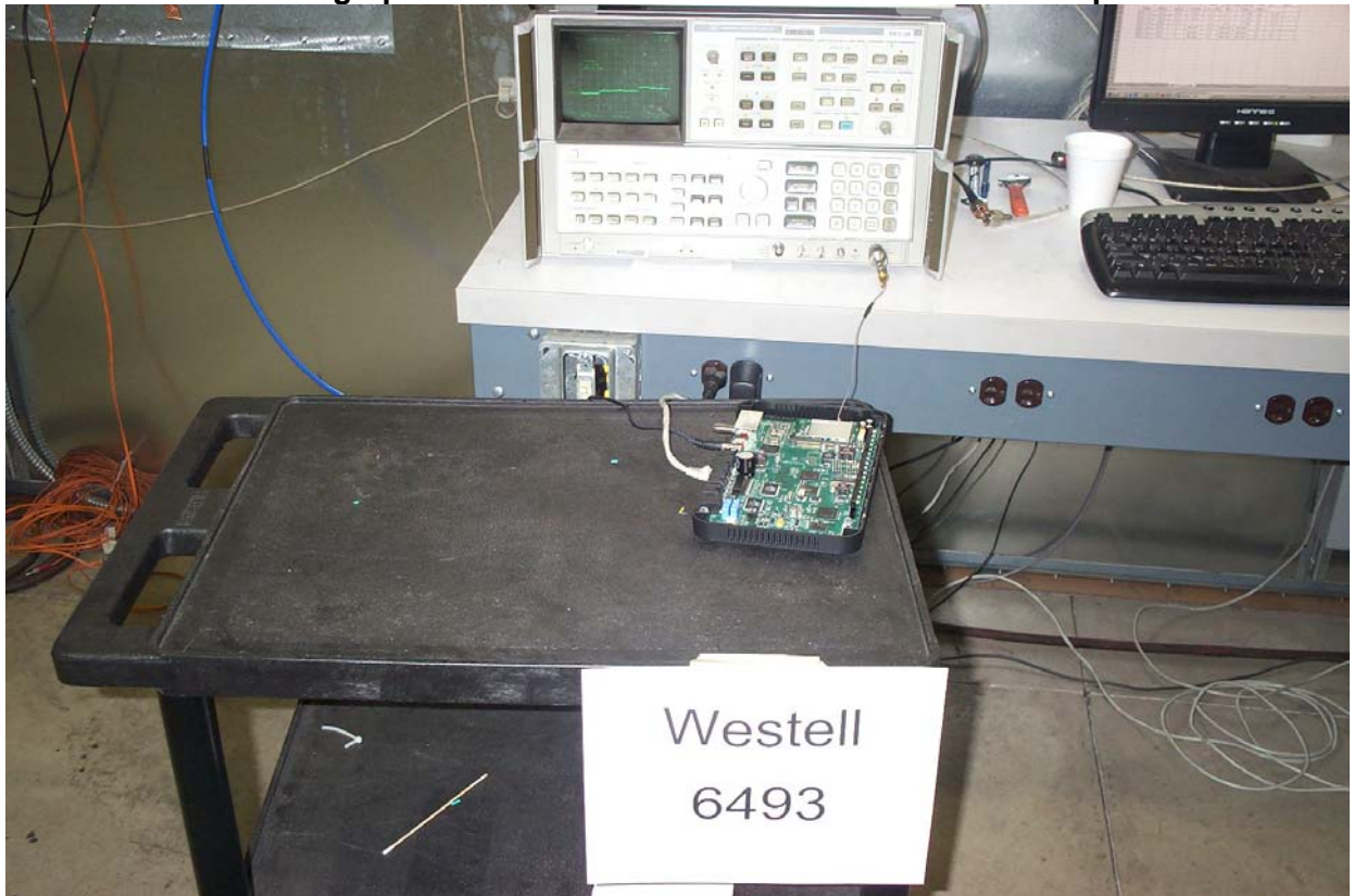
Photograph of Antenna Conducted Emissions Test Setup
