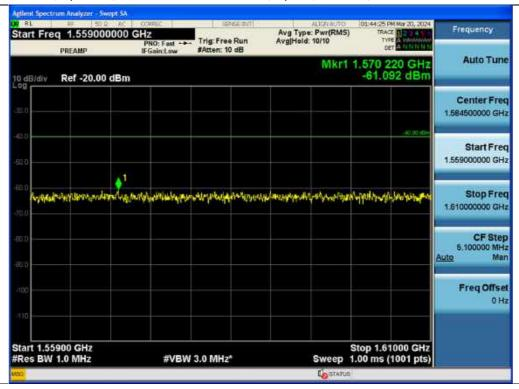
Measured Level + Ant. Gain = -61.092 dBm + 11 dBi = -51.092 dBm(E.I.R.P.) complies with the limit 27.53(f).
