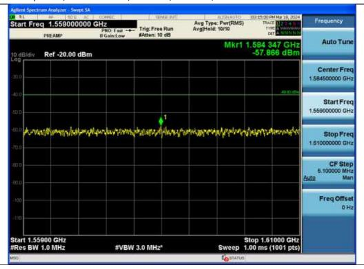
Measured Level + Ant. Gain = -57.866 dBm + 11 dBi = -46.866 dBm(E.I.R.P.) complies with the limit 27.53(f).
