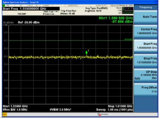
Measured Level + Ant. Gain = -57.894 dBm + 11 dBi = -46.894 dBm(E.I.R.P.) complies with the limit 27.53(f).
