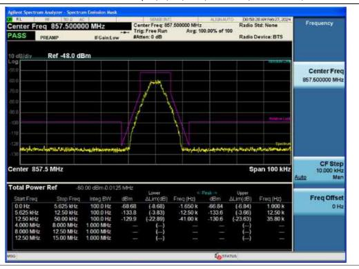
3 dB above the AGC threshold Input / B/ILT; SMR / Downlink / P25 Phase 1 / Mask D
