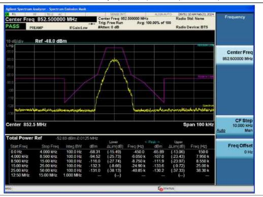
3 dB above the AGC threshold Input / NPSPAC / Downlink / P25 Phase 1 / Mask H
