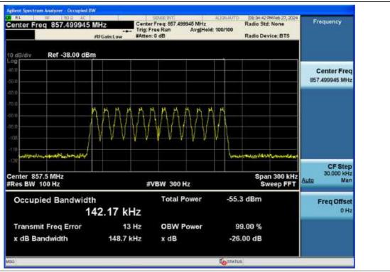
Output / B/ILT; SMR / Downlink / 150 kHz
