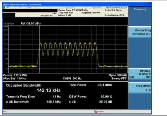
Output / B/ILT; SMR / Uplink / 150 kHz
