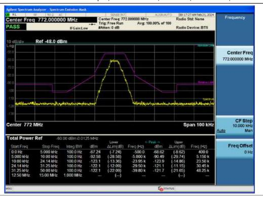
3 dB above the AGC threshold Input / PS Narrowband / Downlink / P25 Phase 1 / Mask C
