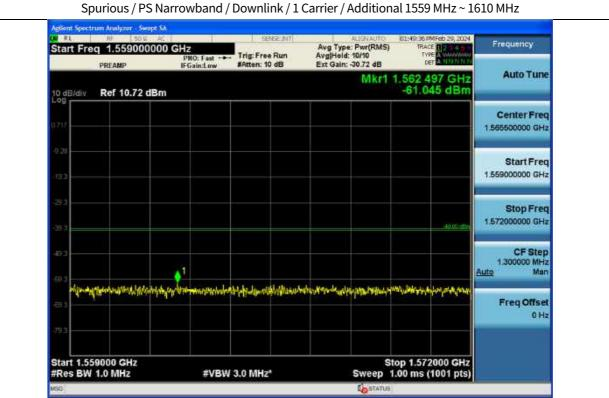
Measured Level + Ant. Gain = -61.045 dBm + 11 dBi = -50.045 dBm(E.I.R.P.) complies with the limit 27.53(f).
