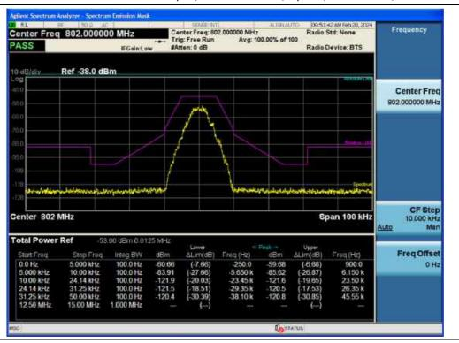
3 dB above the AGC threshold Input / PS Narrowband / Uplink / P25 Phase 1 / Mask C
