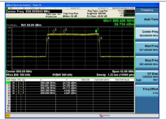
**Note:** The EUT amplifies the frequency range of 851 MHz ~ 869 MHz, but the testing was performed only for the frequency range of 851 MHz ~ 861 MHz. The result of marker 1 is irrelevant.
