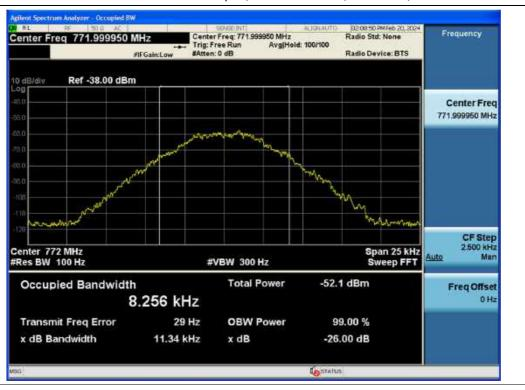
3 dB above the AGC threshold Input / PS Narrowband / Downlink / 12.5 kHz
