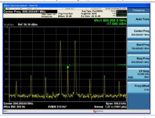
Out-of-band (two adjacent test signals) / PS Narrowband / Uplink
