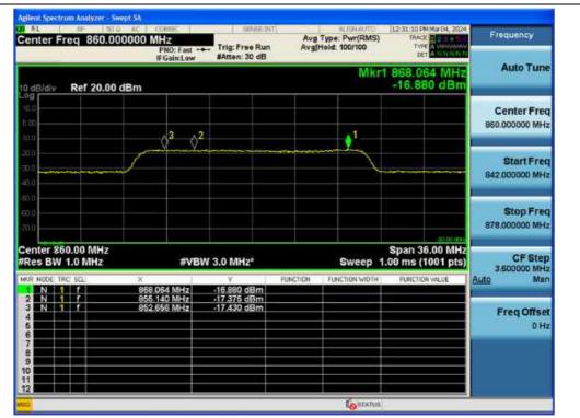
Note: The EUT amplifies the frequency range of 851 MHz ~ 869 MHz, but the testing was performed only for the frequency range of 851 MHz ~ 861 MHz. The result of marker 1 is irrelevant.
