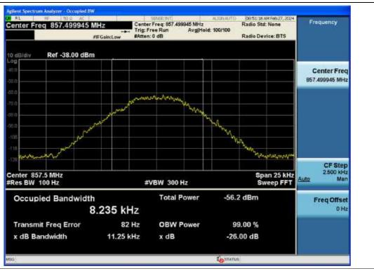
Output / B/ILT; SMR / Downlink / 12.5 kHz
