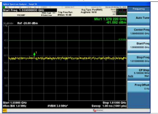
Measured Level + Ant. Gain = -61.092 dBm + 11 dBi = -51.092 dBm(E.I.R.P.) complies with the limit 27.53(f).
