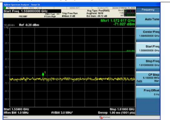
Spurious / PS Narrowband / Uplink / 1 Carrier / Additional 1559 MHz ~ 1610 MHz
