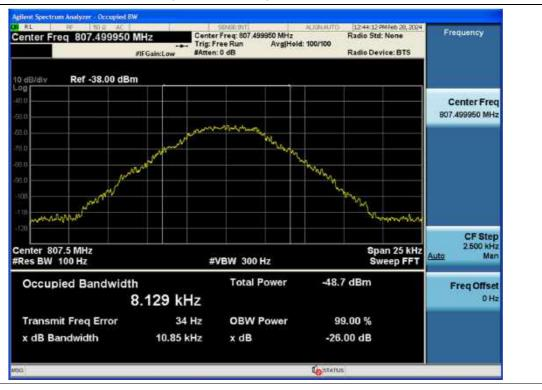
Output / NPSPAC / Uplink / 12.5 kHz
