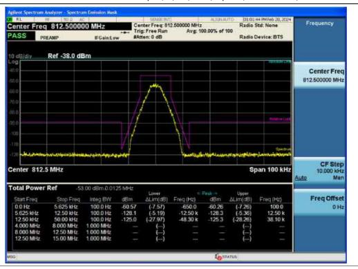
3 dB above the AGC threshold Input / B/ILT; SMR / Uplink / P25 Phase 1 / Mask D
