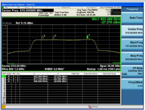
Note: The EUT amplifies the frequency range of 806 MHz ~ 824 MHz, but the testing was performed only for the frequency range of 806 MHz ~ 816 MHz. The result of marker 1 is irrelevant.
