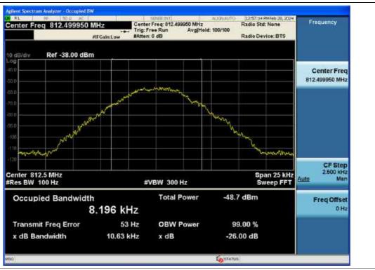
Output / B/ILT; SMR / Uplink / 12.5 kHz
