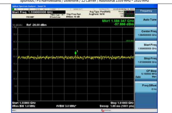
Spurious / PS Narrowband / Downlink / 12 Carrier / Additional 1559 MHz ~ 1610 MHz
