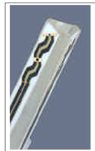
Inside view of ET3DV6 E-field Probe
