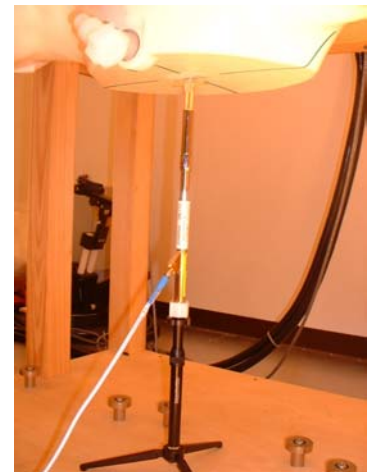
2450MHz System performance check setup
