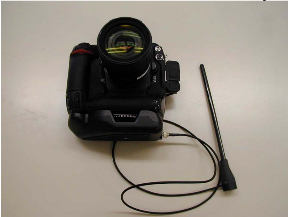
Digital Camera with W-LAN Transmitter & Antenna (WA-E1)
