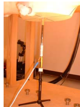
2450MHz System performance check setup
