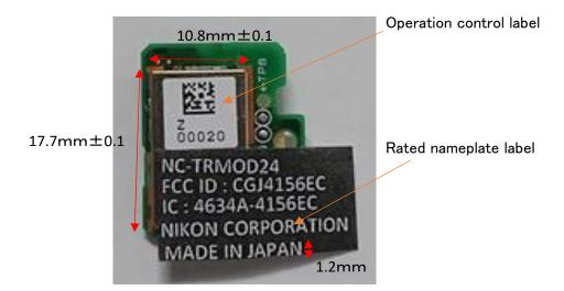
From the figure, it is not possible to attach the process control label and the rated nameplate label at the same time.
