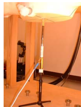
2450MHz System performance check setup
