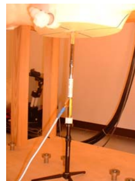
2450MHz System performance check setup
