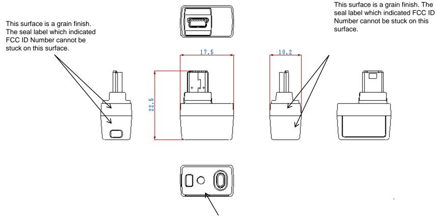
This field has the lens for LED, the WPS button, and a hole for straps. There is no space which indicates FCC ID:CGJ2148EA.
