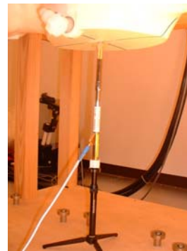
2450MHz System performance check setup
