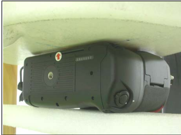
A: The bottom of the EUT face to the phantom with 0mm-separation distance.
