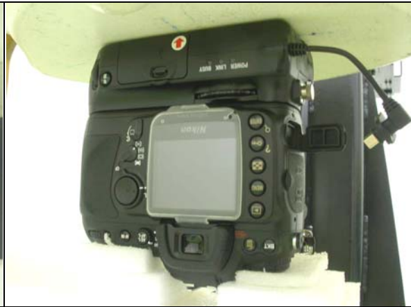
B: The edge of the EUT face to the phantom with 0mm-separation distance.
