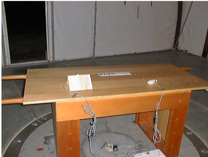
Figure 6.16 - Radiated Emissions, Open Area Test Site (NX1700E)
