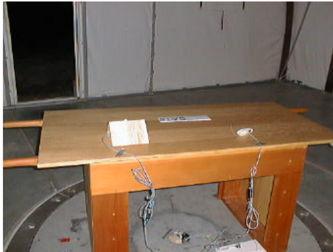
Figure 6.16 - Radiated Emissions, Open Area Test Site (NX1700E)
