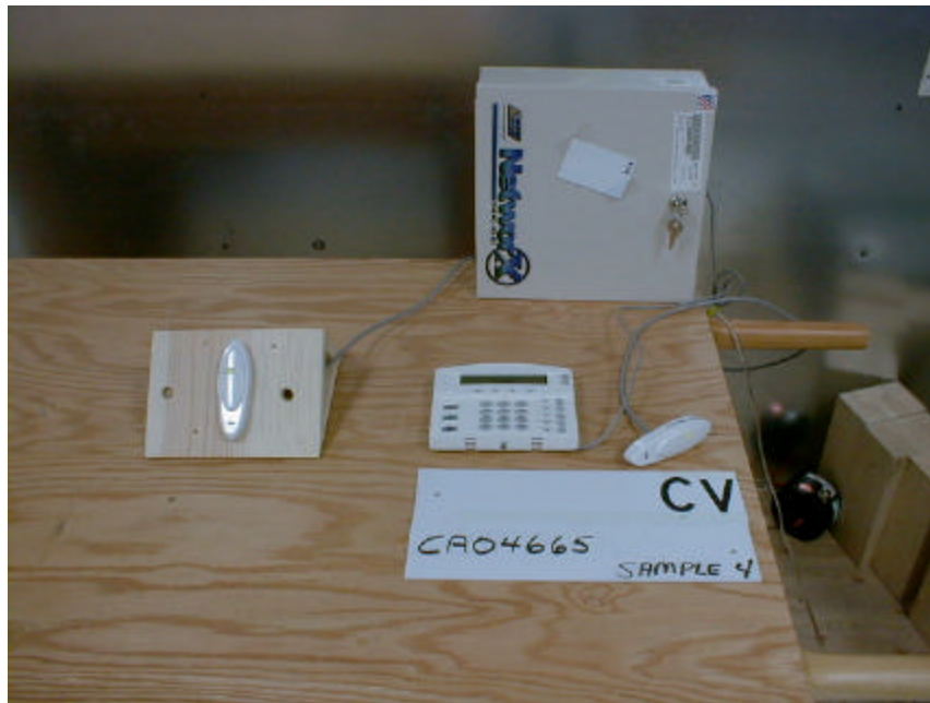
Figure 6.10 - Conducted Voltage Emissions Measurement Configuration (NX-1700E)
