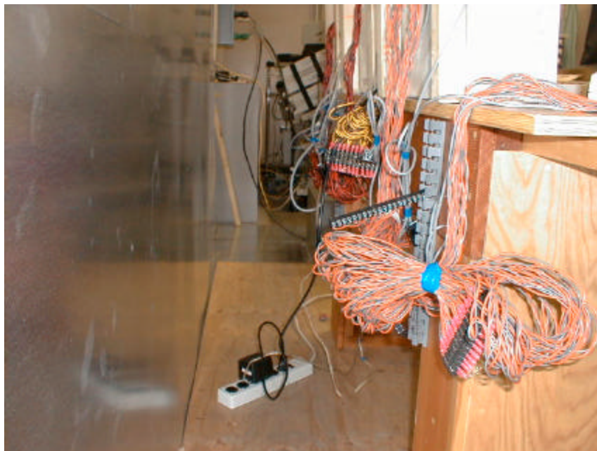
Figure 6.9 - Conducted Voltage Emissions Measurement Configuration (AL-1193)
