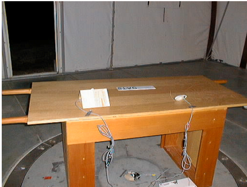
Figure 6.20 - Radiated Emissions, Open Area Test Site (NX1700E)
