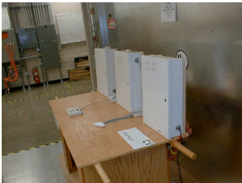
Figure 6.2 - Conducted Voltage Emissions Measurement Configuration (AL-1191)
