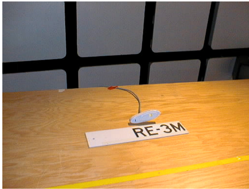
Figure 6.16 - Radiated Emissions, Pre-scan, 3m Chamber (NX1700E, AL-1191 and AL-1193)
