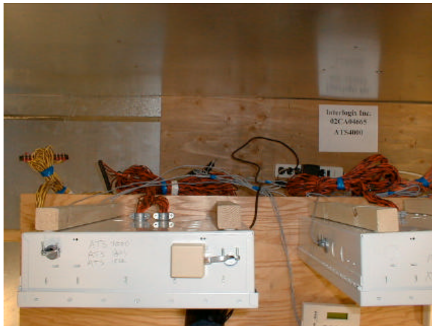
Figure 6.6 - Conducted Voltage Emissions Measurement Configuration (AL-1191)
