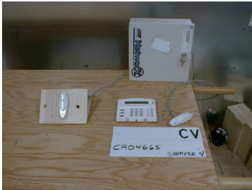
Figure 6.5 - Conducted Voltage Emissions Measurement Configuration (NX-1700E)
