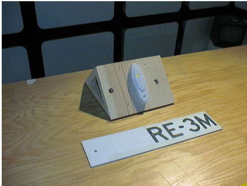
Figure 6.10 - Radiated Emissions, Precompliance, 3m Chamber
