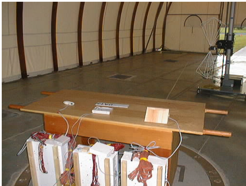
Figure 6.14 - Radiated Emissions, Open Area Test Site (ATS-1190 and 1192)
