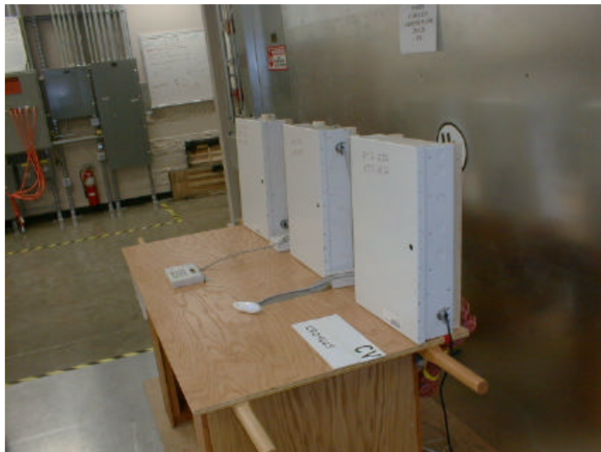
Figure 6.2 - Conducted Voltage Emissions Measurement Configuration (ATS-1190)
