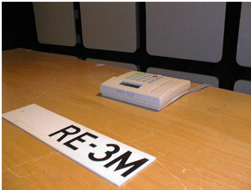
Figure 6.8 - Radiated Emissions, Precompliance, 3m Chamber
