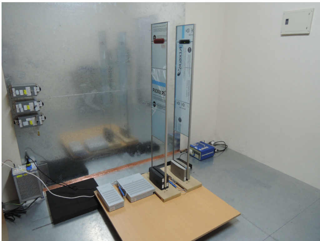
Photograph 5: Set-up for for Mains Conducted testing Front
