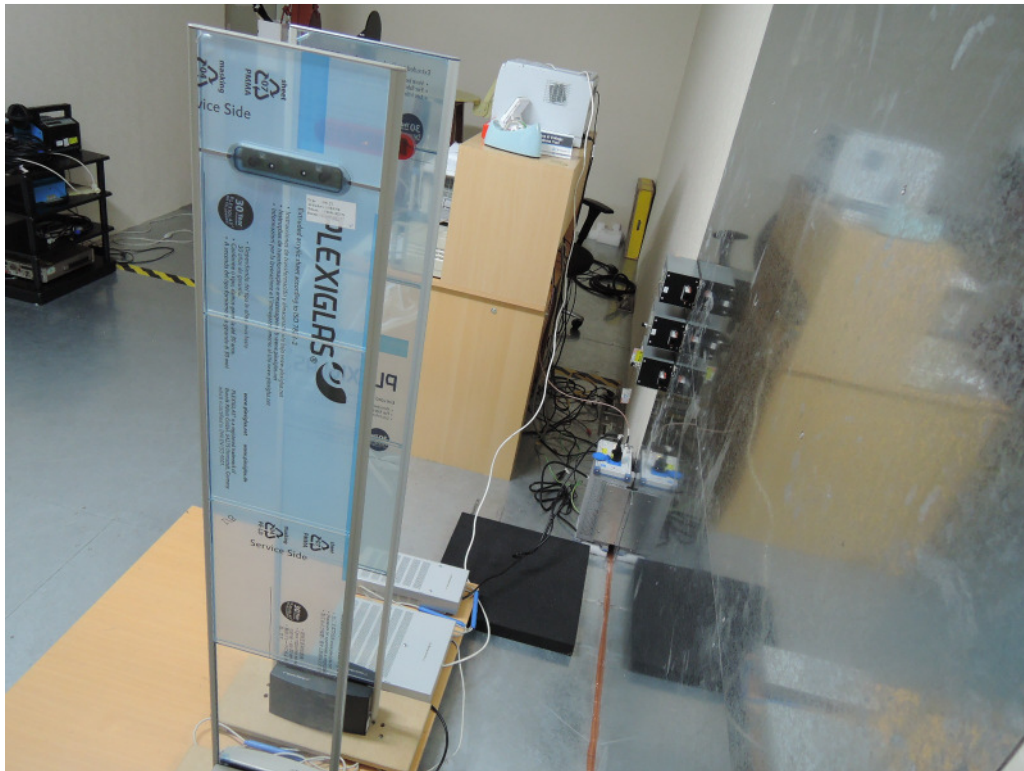
Photograph 4: Set-up for for Mains Conducted testing Back
