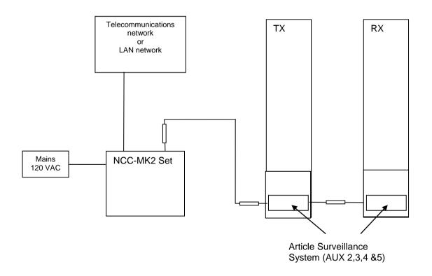
Figure 1: Basic testsetup and connections
